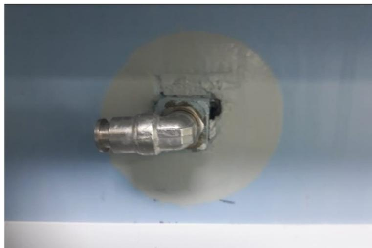
*Figura 7 – ITEM 7: COTOVELO TUBO 08 X ROSCA MACHO ¼ BSP (CONEXÃO PNEUMÁTICA METÁLICA)*
